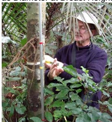
**Using a diameter tape:** A diameter tape is supplied with FORMAK. Diameter tapes have a scale that allows diameter to be read directly when the tape is wrapped around the circumference of a stem. In the image below, diameter is measured as 143 mm.
