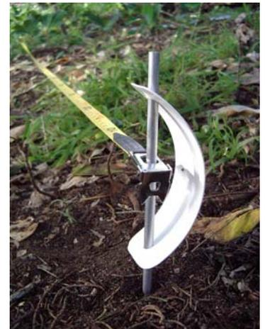
12 Peg the plot at the 20m mark. Wrap the tape around the 20m plot peg to secure it so that the tape is firm, but able to follow the ground profile (i.e not stretched across a gully well above the ground)
